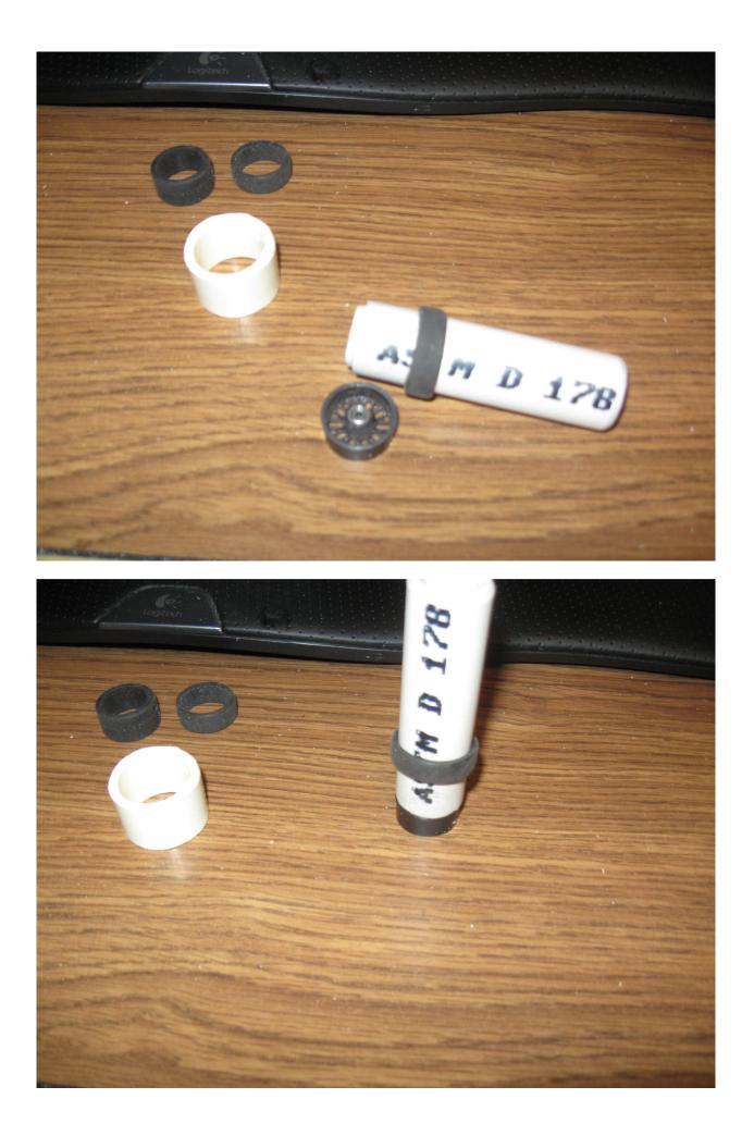
The next part is a  $\frac{3}{4}$ " collar. These have a stop in the middle that centers the collar on each piece of pipe when used for its intended purpose. This stop must be removed which was done with the Dermal used before. In my case I cut this part in half for reasons shown below.
