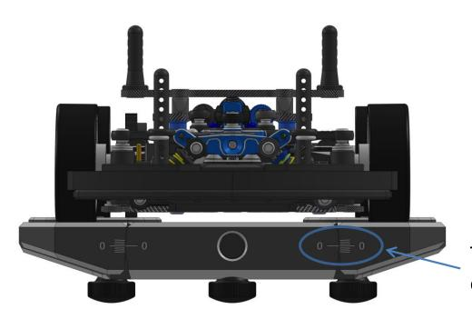
Try to align marking with zero based on the below procedure 6.2.
